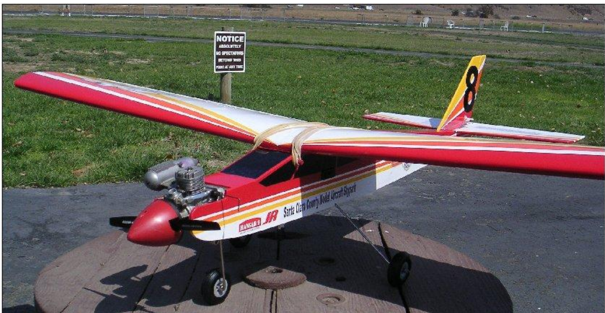
Hangar 9 Alpha powered by an OS 46 SX 2-stroke. Mike French photo.
