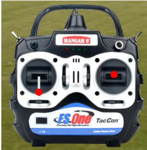
Figure 1. Controls at engine idle (left stick) and neutral (right stick).
