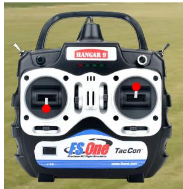
Figure 4. Right control stick pushed forward—plane pitches down.
