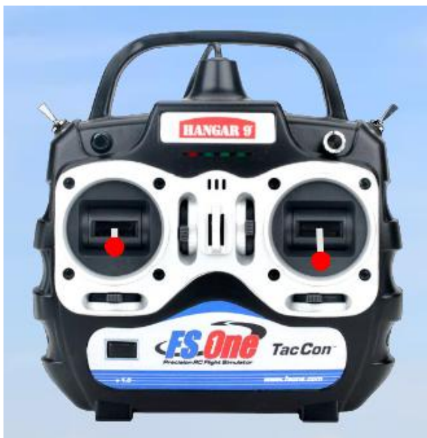
Figure 3. Right control stick pulled back—plane pitches up.
