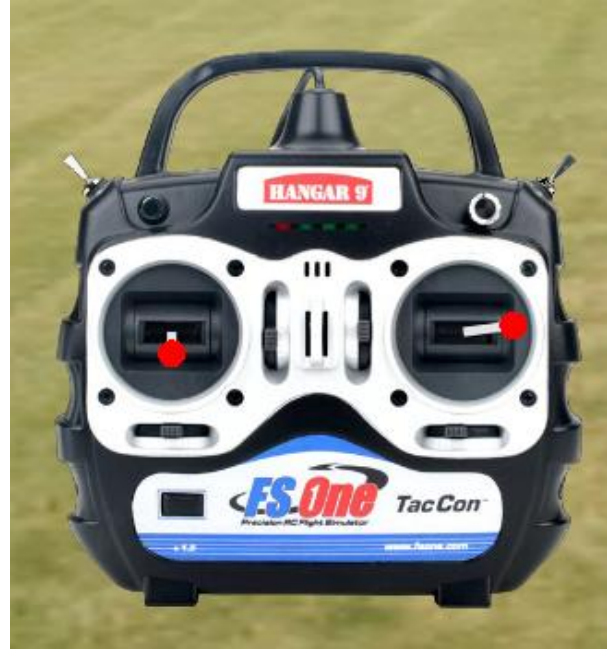
Figure 6. Right control stick moved right. Plane banks right.
